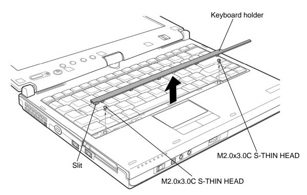
Figure 4-14 Removing the keyboard holder
